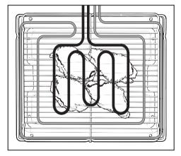
For grilling small quantities of thin cuts and for browning small dishes of food. The inner part of the grill element is switched on and glows red.
